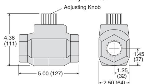
**Operation:** To increase flow: Turn adjustment screw out.
